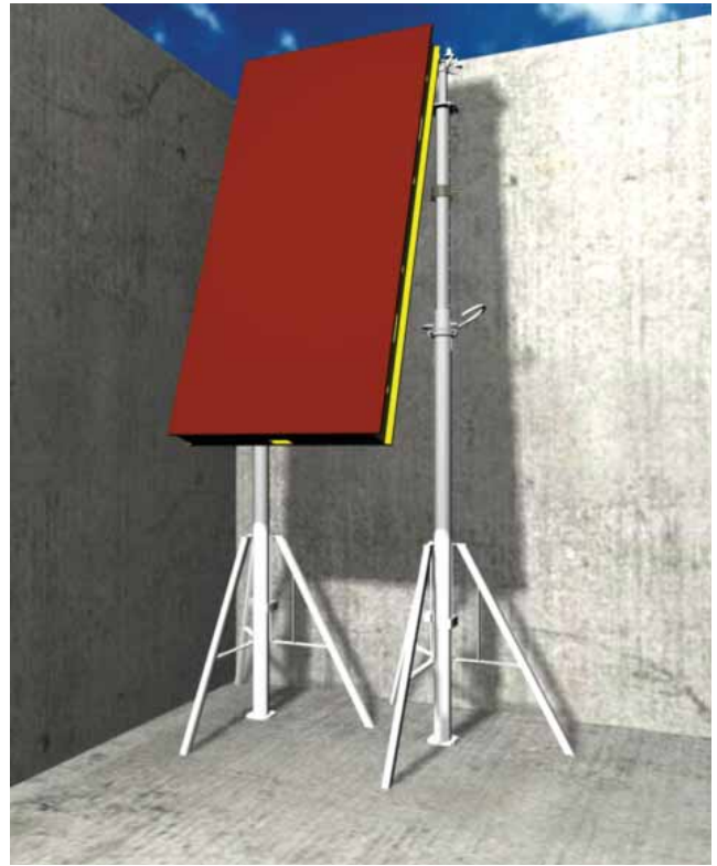
B. Hang the Alu Top Deck panel onto the Top Deck Bearing as illustrated. If the panel is properly placed, the cams of the bearing devices will hold the panel.
