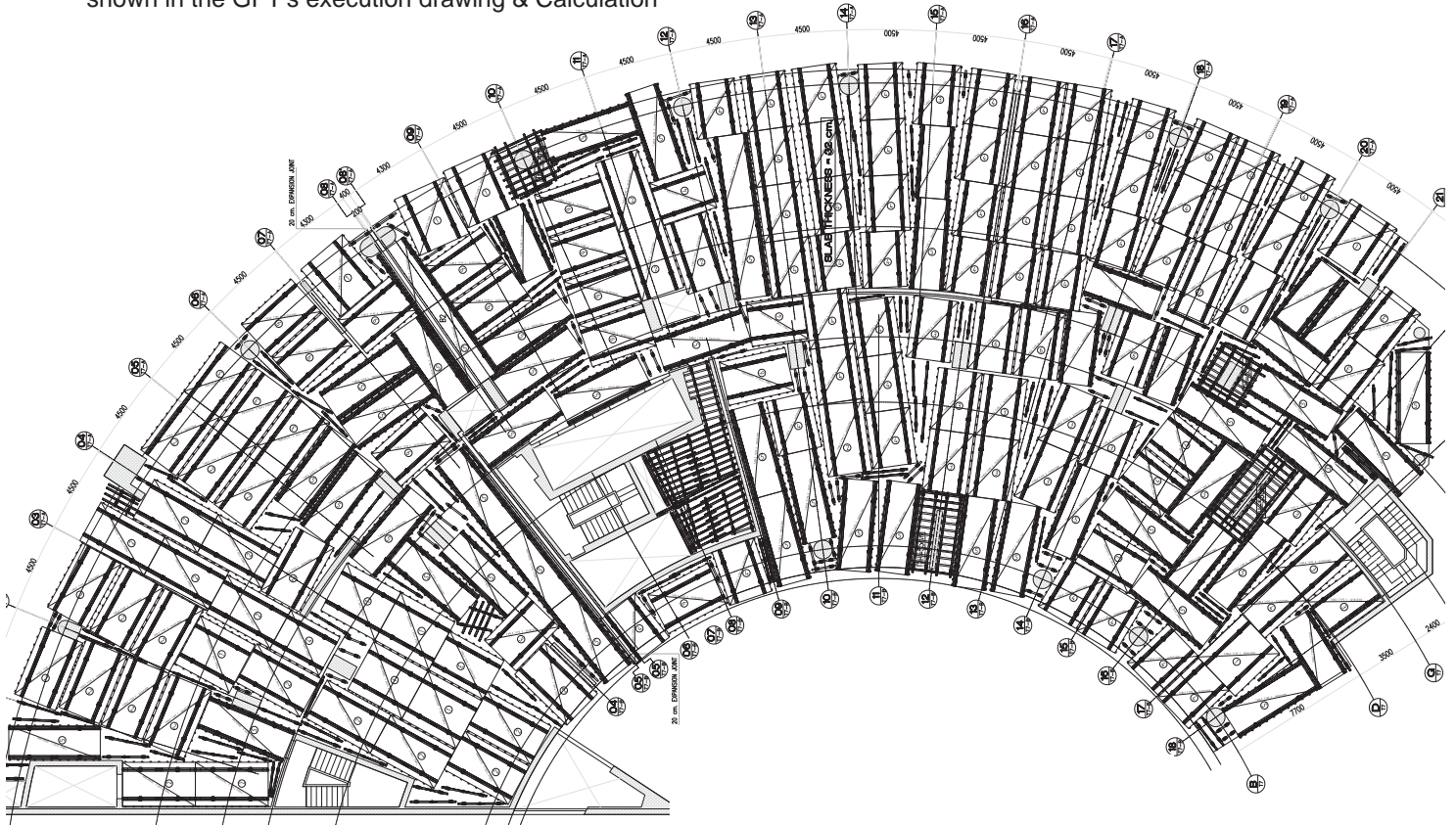
Formwork Layout using H20 Slab Table System
